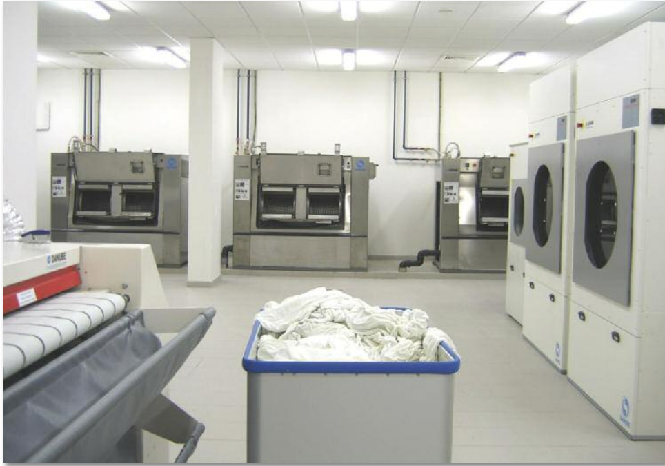
HOTEL HYGIENE: More hotels are installing barrier washers, the CS washers are seen here at the Galynish Hotel Academy
